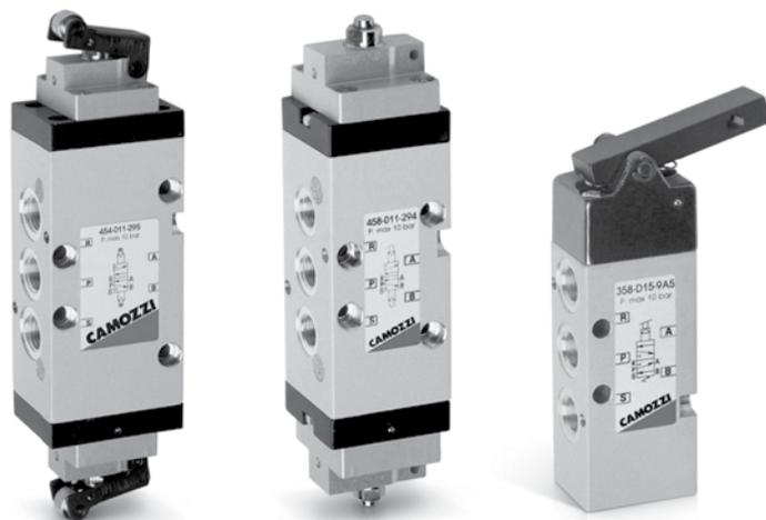
In order to facilitate the use of limit switch valves in applications where very low actuating forces and high flow rates are required, the Series 3 and Series 4 valves are equipped with new mechanical devices designed for this purpose. The Series 3 valve is designed with a mechanical lever which when operated releases an internal pilot signal to atmosphere. Actuation forces are less than 50g and the sensitivity can be increased by adding a "whisker" or rod of dia. 3mm to the lever.
