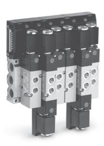
This Plug-In system based on the electropneumatically operated valves Series 3, G1/8 delivered completely assembled and tested, can accomodate up to 22 valve positions (with two SUB-D connectors), has a protection class of IP 65. The electrical part is based on printed circuit boards.
