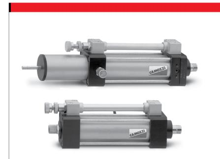
The Series 43 hydrocheck units are available with two different types of control: regulated outward movement and fast return; or fast outward movement and regulated return. These hydrochecks come complete with an oil surge tank which ensures automatic equalization.
