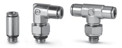
Micro Super-Rapid fittings are constructed in 14 different models. Connection and disconnection of the tube, can be repeated several times and can be performed using one hand and without the use of tools. The sealing ring (O-Ring) can be easily replaced if it is damaged or should the rubber compound from which it is made wear with time.
