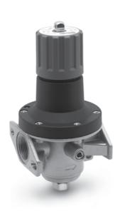
This valve is designed so that the downstream air pressure can be vented and the valve locked in the non passing condition to allow the work to be carried out with greater safety on pneumatically actuated equipment.
