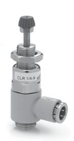
Series CLR micro pressure regulators are available with G1/8 and G1/4 connections. A piston with relieving and VS function (valve with fast draining) has been incorporated into its design. The body is in brass, while the connection fitting is in technopolymer which guarantees maximum lightness. With a threaded top part of the body both direct mounting to a valve outlet (1/8 and 1/4 threads) and panel mounting are easily facilitated.
