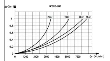
Flow diagram for model: MC202-L00
