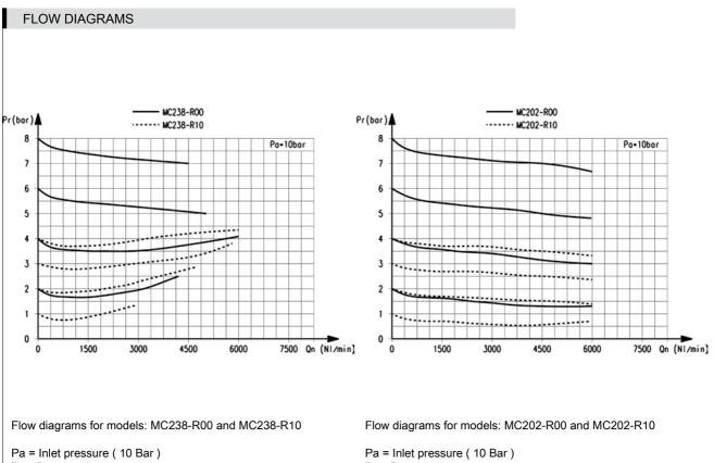
Pa = Inlet pressure (10 Ba Pr = Regulated pressure Qn = Flow Pa = Inlet pressure (10 Bar) Pr = Regulated pressure Qn =Flow
