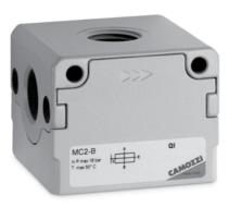
The take-off blocks when equipped with a no return valve, allow the use of non lubricated air and should be inserted between the regulator and the lubricator. If mounted as last element, they should be assembled with terminal flanges.
