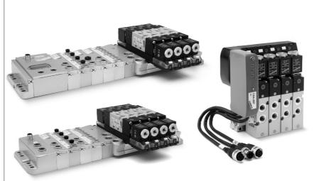
The Multipole version of Series 3 Plug-In valve island can be easily installed thanks to the front position of the Sub-D connector. The accessories of the new connection system to the Series CX serial nets enable to handle up a multipole valve island by means of a Sub-D connector or through a node integrated in the island. The modularity of the electric and pneumatic parts allows to install up to a maximum of 22 solenoids on 22 valve positions.
